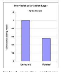
Interfacial polarization conductance scaling factor for an unfouled and foulded RO membrane.
