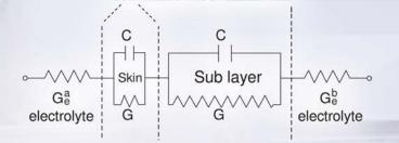
The equivalent circuit for a membrane containing two such substructural layers in contact with an aqueous electrolyte.
